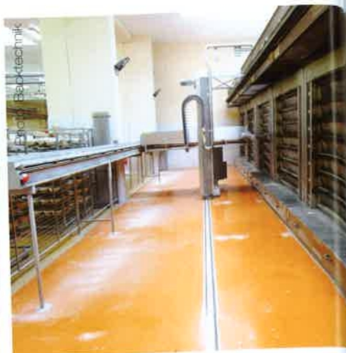
Left photo: The automatic bread line also includes a fermentation cabinet in which the dough can relax and ferment. Middle photo: The pre-fermented breads are put on a transfer table which forms the interface to the oven loader. Right photo: Five multi-deck ovens with a baking surface of 26 square metres each are available for the production of the range of breads.
