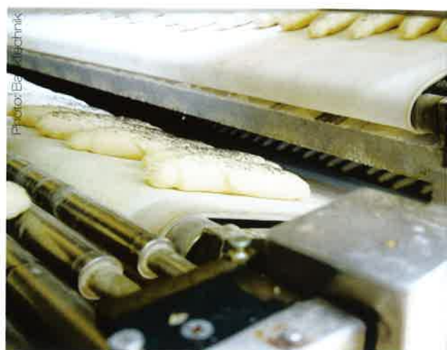
Left photo: Before the oven, the Rohliks are moistened over the whole width of the line, i.e. 30 products per row. Right photo: A variable switch feeds the upper and the bottom part of the oven by turns. If necessary, it can also feed only one hearth with products.
