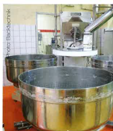
Left photo: A conveyor belt, where the products can cool down, guides the products to the counter where they are put in baskets. Middle photo: The quality of the products has been improved clearly with the purchase of the new tunnel oven. Right photo: A kneader carousel with three bowls made by the Italian manufacturer Mixer feeds the bread line with dough.
