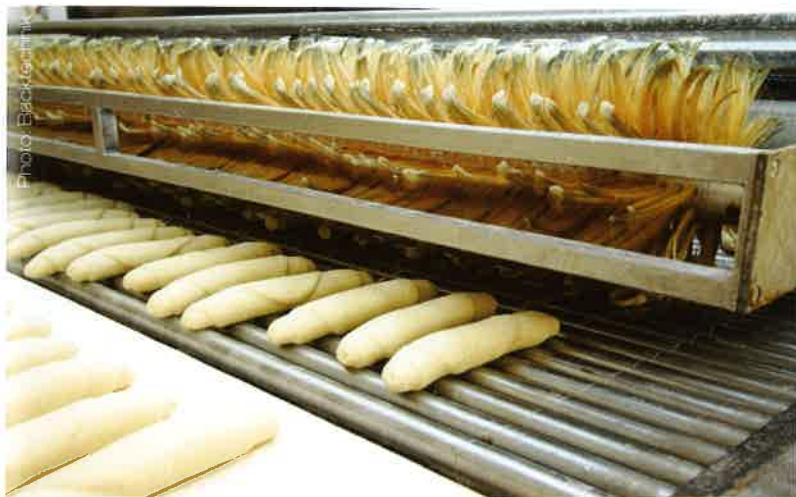
Left photo: Before the oven, the Rohliks are moistened over the whole width of the line, i.e. 30 products per row. Right photo: A variable switch feeds the upper and the bottom part of the oven by turns. If necessary, it can also feed only one hearth with products.
