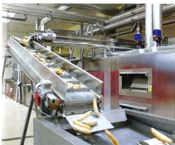
Left photo: A conveyor belt, where the products can cool down, guides the products to the counter where they are put in baskets. Middle photo: The quality of the products has been improved clearly with the purchase of the new tunnel oven. Right photo: A kneader carousel with three bowls made by the Italian manufacturer Mixer feeds the bread line with dough.
