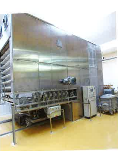
Left photo: The automatic bread line also includes a fermentation cabinet in which the dough can relax and ferment. Middle photo: The pre-fermented breads are put on a transfer table which forms the interface to the oven loader. Right photo: Five multi-deck ovens with a baking surface of 26 square metres each are available for the production of the range of breads.
